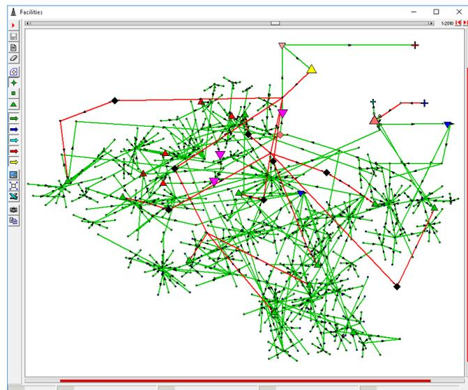
**Identification of Calculation Problems.** Pipes that have not been calculated can be identified. For example, that could be due to the disconnection of nodes from the network.
