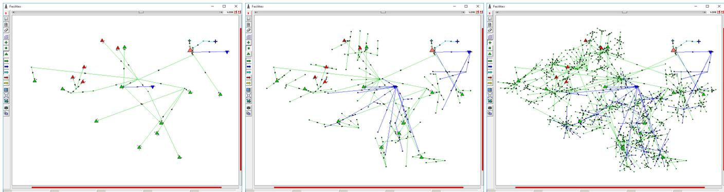
**Visualization Options.** Partial visualization is allowed at different levels of the hierarchy. We see from left to right, first the network at plant level, then at manifold and satellite level, and finally the complete network from wells to delivery point.
