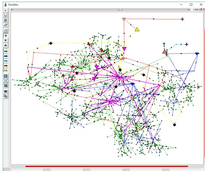
**Associated Nodes.** By selecting a node, all nodes that are upstream or downstream can be identified. The example highlights all the nodes converging to the E-3 Battery.
