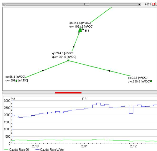
**Display Focused on a Particular Node.** For each node and pipe, specific data such as flow rates or pressures, and production charts
