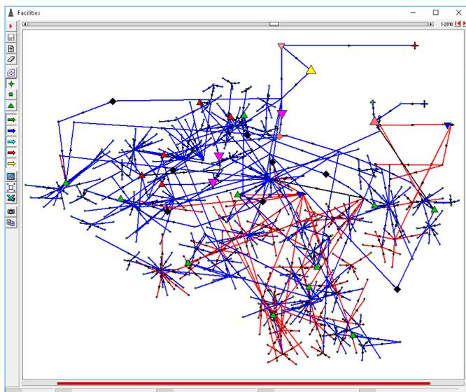
**Identification of High and Low Pressure Zones.** A range of colors can be used to show the pipes depending on the pressure they have. In this example, the range of colors from blue to red characterizes low to high pressures.
