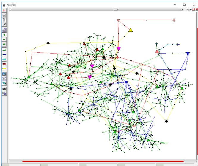
**Identification of the Different Networks.** The liquid production network is shown in green, the gas production network in red, the injection network in blue, and finally the water transference network in light blue if there is an external source.
