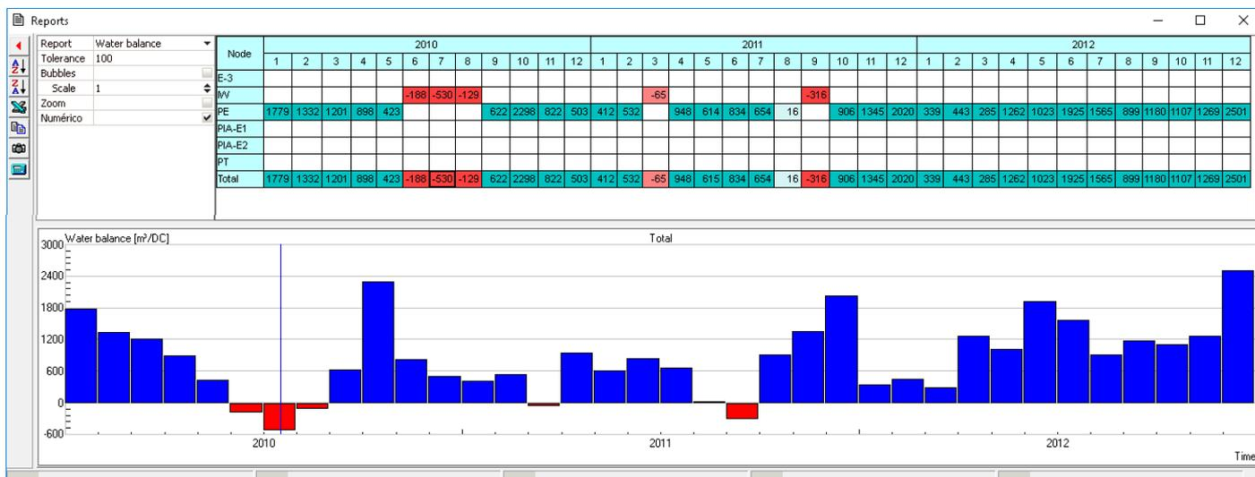
**Water Balance Report.** The movement of water can be observed in those nodes where there is entrance or discharge of water. Months in red show a water deficit. The report can be viewed qualitatively or quantitatively, showing the associated flow rates.
