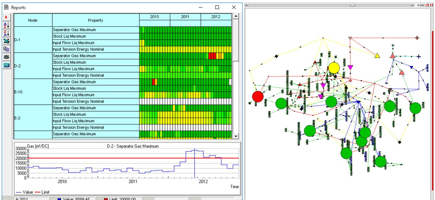
**Capacities Report.** The Properties report shows a range of colors for the properties defined in each of the nodes. Also, bubbles on each node show the selected property and a time chart for the chosen node.
