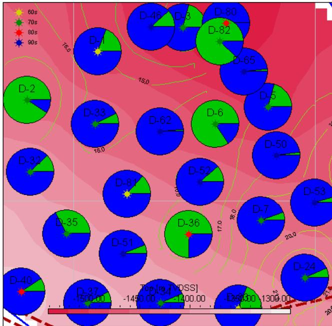
**Map Window.** In this example the structural map is displayed alongside the outlines for net thickness. Additionally, each well is displaying as a pie bubble its proportional water and oil rates for the active date.
