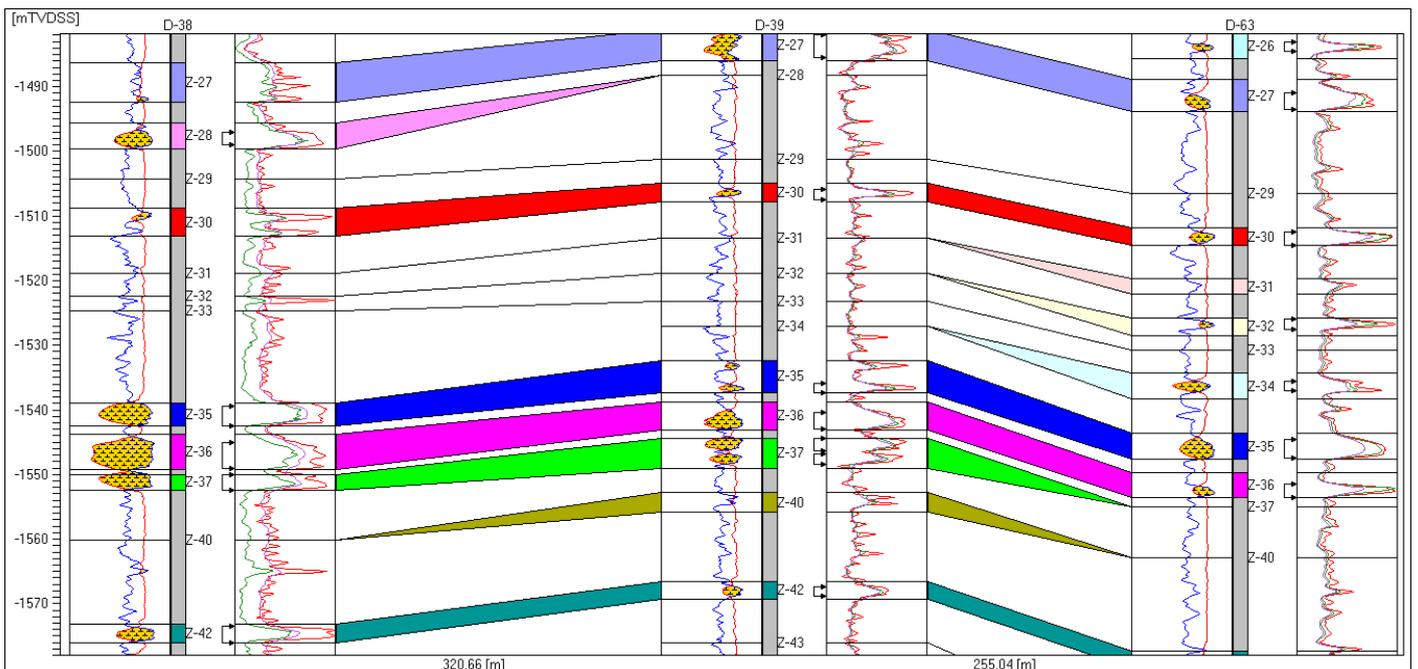
**Cross Sections Window.** A 3 well structural cross section is displayed. For each well, SP and GR logs can be seen, showing productive sands with a shaded area between both curves and the resistivity logs. Additionally, the correlated layers showing their tops and bottoms are visualized. The perforated intervals in brackets give access to the results of the tests performed.
