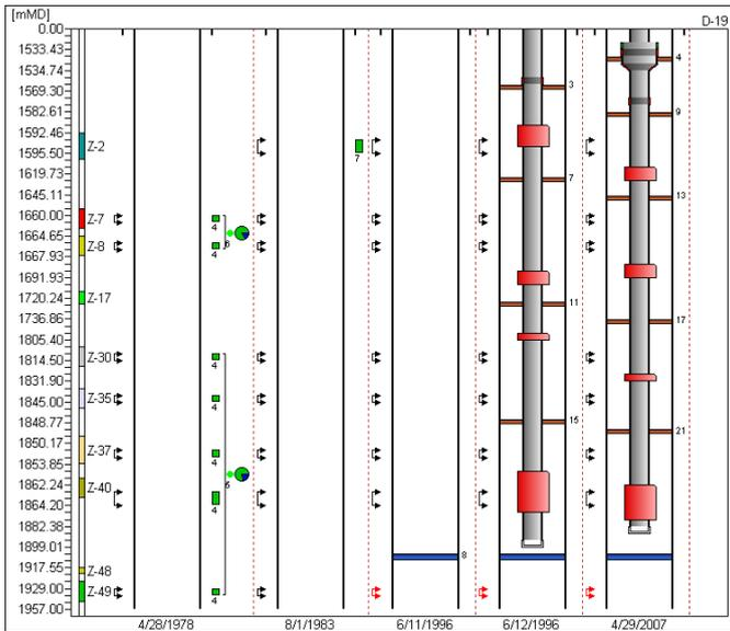
**Wellworks Window.** The wellwork and facility evolution is displayed for an injector well. Perforations, cementations, stimulations and test results can be observed for each date.
