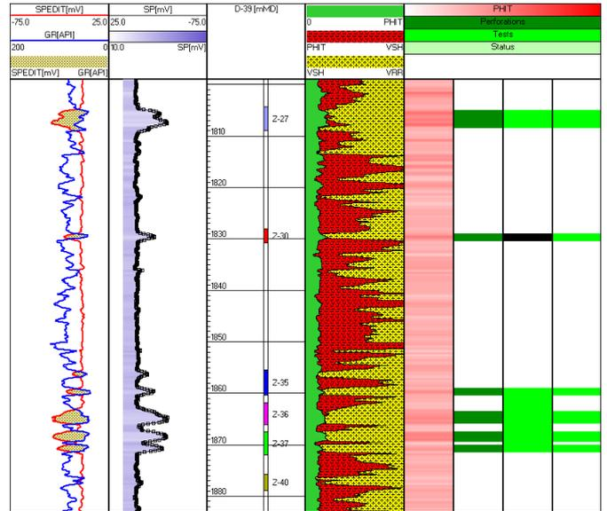
**Logs Window.** In different tracks, electric logs are displayed with highlighted zones, and flags indicating perforated, stimulated and tested zones. The central track shows layer tops and bottoms for the selected well.
